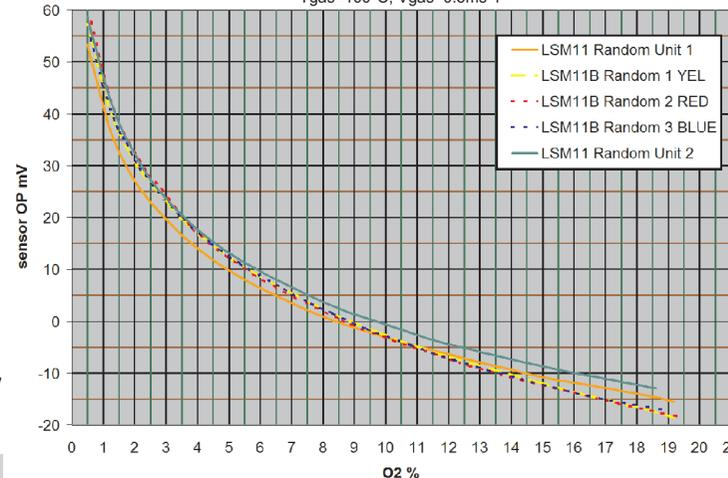
Graph 2 - Demonstration interface design. LSU4.9 (5-wire) vs LSM11B (4-wire, offset and curve corrected to give 0-10V linear output)
