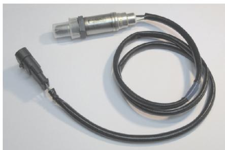
Remove protective plastic cap before fitting. This provides drop protection to the end of the sensor during transit
