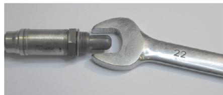
You will require a 22mm open ended spanner for fitment. Make sure the sensor is tightly fitted. If the boss on the flue has a damaged thread it will require replacement. Hand tools only, 60Nm is OK. Metal washer will be crushed slightly during tightening to form a seal
